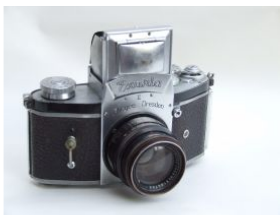
Kine-Exakta II, 1949, body no. 653045. Bottom embossed: "Made in Germany". Fitted with 5.8cm f/2 Carl Zeiss Jena Biotar. Note the curious little accessory bridging the flash points on the left, providing a concentric contact (PML)
