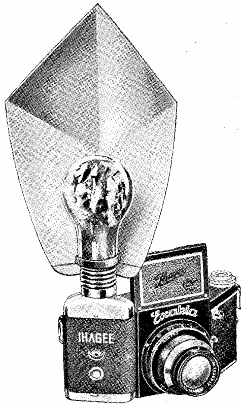
Vacublitz flashgun fitted to a Standard Exakta. It was supported solely on two contact pins until a third, screw pin, was added for security.
