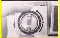
6. A special setting of the frame counter is not necessary since the latter, springing automatically back as soon as the camera back is opened, will begin to operate when the camera back is closed. -Afterwards the frame counter will indicate the number of photographs already taken on the Illm placed in the camera.
