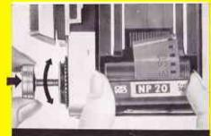
2. Place the cassette containing the unexposed film in the cassette chamber (28). Push the knob of the rewind crank (14) backwards, twisting it gently: the carrier of the rewind arbor (27) must engage with the cassette core.
