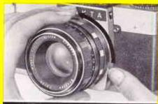
Changing the lens (22): Press the locking lever (19) towards the lens. Then turn the lens to the left until the orange-coloured dots (12 and 13) are in line. Lift the lens out towards the front. — To insert a lens, proceed in the reverse sequence: line up the orange-coloured dots, and turn the lens to the right until it locks in place.
