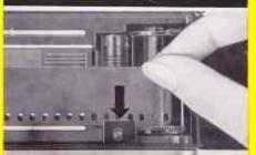
3. Pull the beginning of the film (29) as far as the green mark (35), and push it with its (lower) perforation from above under the film rest (33) and, accordingly, over the film-wind sprocket (32). The catch bow of the take-up spool (34) must not stand upwards!
