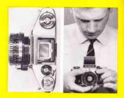
the camera must be held close to the eye. When taking vertical pictures with the Finder Hood it is possible to shoot at right angles. This is particularly useful for working inconspicuously since the photographer can remain in concealment. (The Penta Prism makes it possible to the process of the process of the process of the prism makes it possible to the prism makes it
