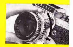
3. Changing the lens (28) (select autmoatic on all lenses from Jena): depress the locking lever (30) towards the lens, then turn the lens to the left until the two red dots (23 and 29) are in line, and lift the lens out towards the front. To insert a lens proceed in the reverse sequence: line up the red dots, and turn the lens to the right until it locks. All special-purpose lenses can be used with focal lengths ranging from the shortest, to the longest.
