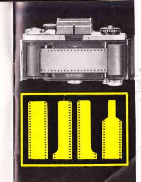
It is not necessary to trim the beginning of the film specially. Any shape of leader can be used with the take-up spool of the EXAKTA VX 1000, either the narrow tongue provided on standard commercial cassettes, or, even better, a straight cut-across end as obtained when cutting lengths of film from bulk rolls. When employing a take-up cassette the film must be trimmed to suit the core of the cassette spool.
