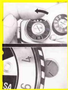
10. Setting frame counter (6). Turn the disc of the frame counter (6) with the index finger to the left (anti-clockwise), until, when using a film with 36 exposures the figure "36", or when using a film with 20 exposures the figure "20" appears in the centre of the window.
