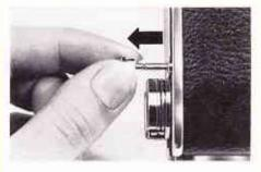
cutting knife (37): Withdraw the knob (38) about 13/4 inches from the comera body. Then press the knob (38), returning it to its rest position. Wind on, and expose two blank frames, in order to draw the end of the film across into the take-up cassette.
