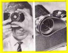
should use their distance glasses for focusing with the Penta Prism. Refer to page 38 for instructions on the use of the Fresnel screen. – For fitting and removing the Penta Prism see page 39. An invaluable accessory for use with the Penta Prism is the flexible eyepiece cup:
