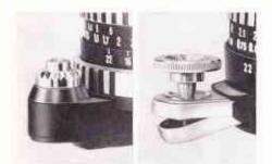
For all exposure times of 1/s sec. or longer, or exposures using the delayed action, lenses having automatic diaphragms should be set to manual in order to avoid premature opening of the aperture. When using the Domiplan 2.8/50 lens, a cable release with a long plunger and time-exposure lock, or the special locking knob (available as an accessory) should be employed for the release rocker. For more information regarding this, see the detailed description of lenses on pages 28-31.
